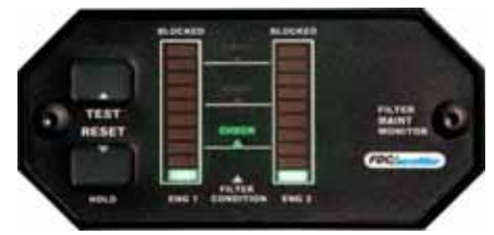
fig. 1 - lamps indicate a clear filter
