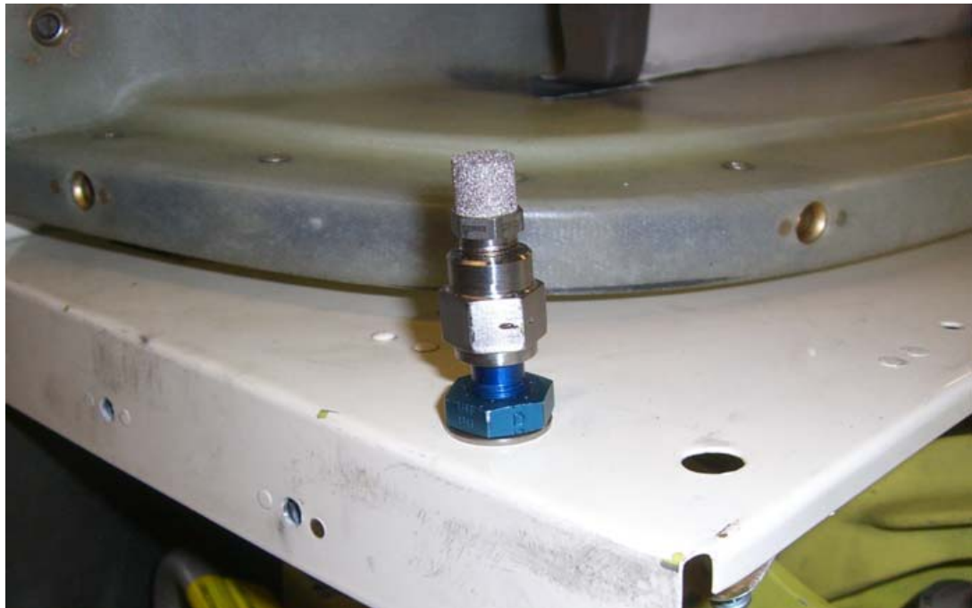
Figure 6 – Static Port Installation
