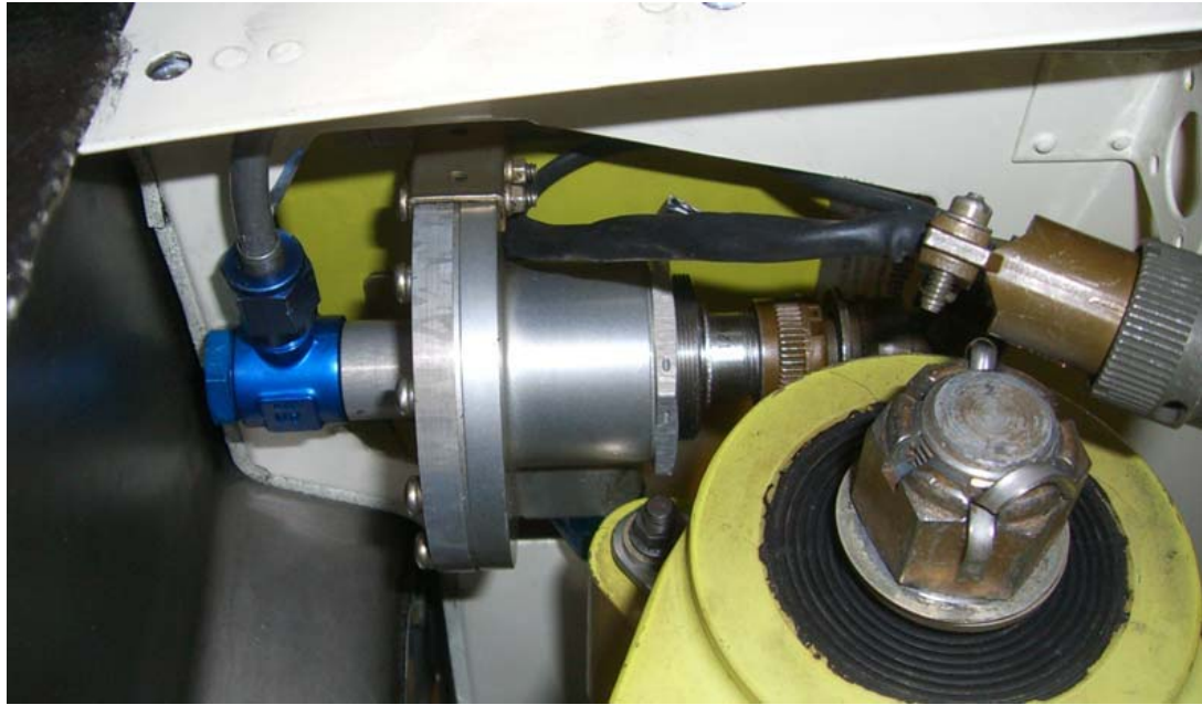
Figure 5 – Differential Pressure Switch Installation with Banjo Fitting
